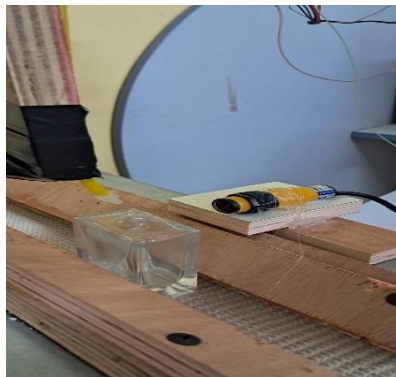
Figure 4.6: IR sensor installed on the conveyor for bottle detection
