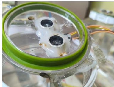
Figure 4.7: Ultrasonic sensor mounted above the ingredient tanks
