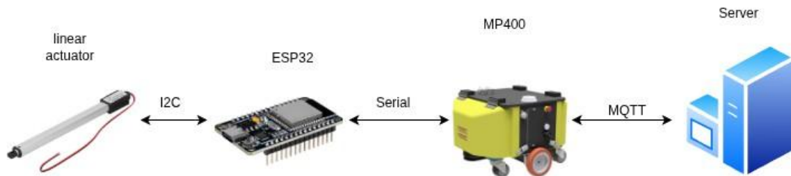
Figure 2.1: Hybrid Edge–On-Premises Architecture
