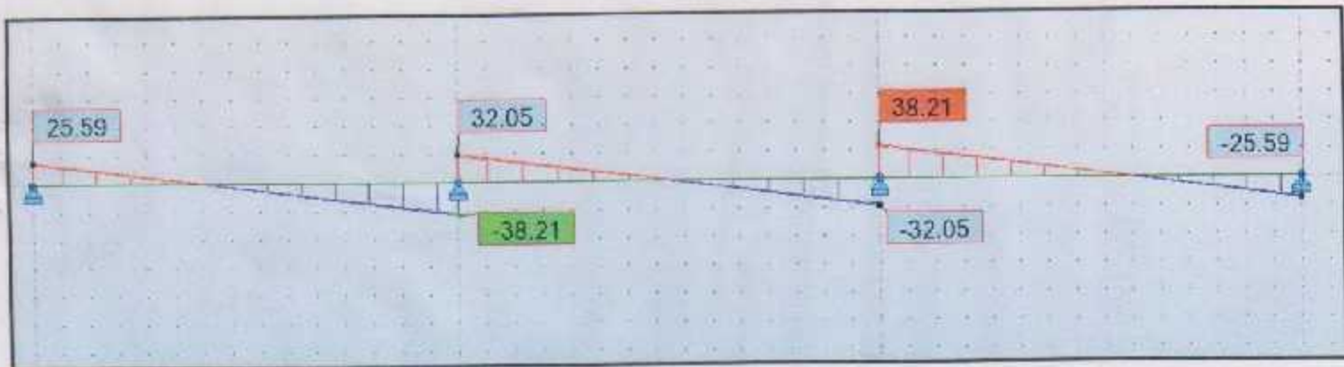
Figure (4-3): System of slab of parking shed with loads
