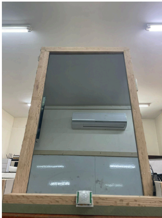
Figure 4.7: The smart mirror with the wooden frame and two way glass
