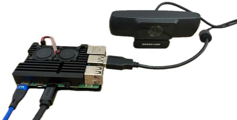
Figure 4.1: Webcam camera connected to Raspberry Pi 4.
