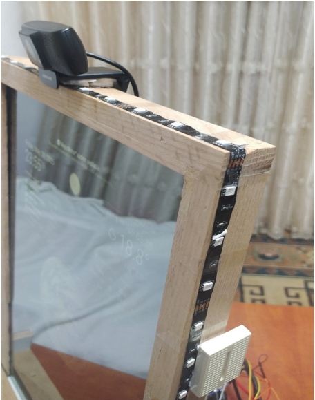
Figure 5.3 : RGB Led Strips in light
