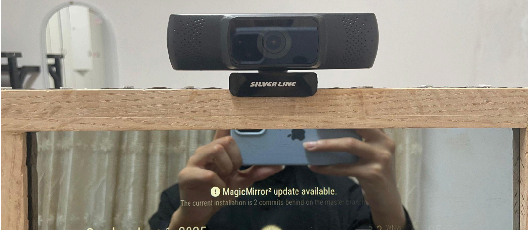
Figure 5.4 : USB Webcam placement on the mirror.
