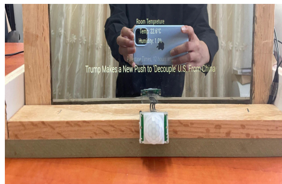
Figure 5.12: The PIR sensor on the mirror
