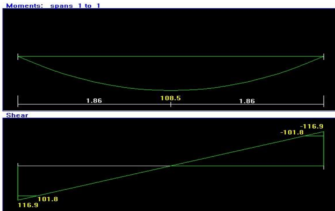
Figure 4. 11: Moment /Shear Envelope of basement wall
