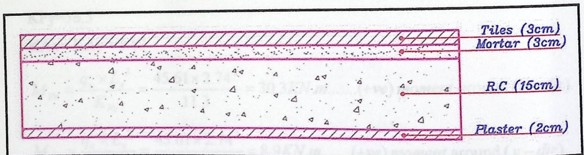
Fig.(4.42): section in stair's landing
