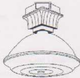
FIGURE 3.4 Enclosed metal halide luminaire
