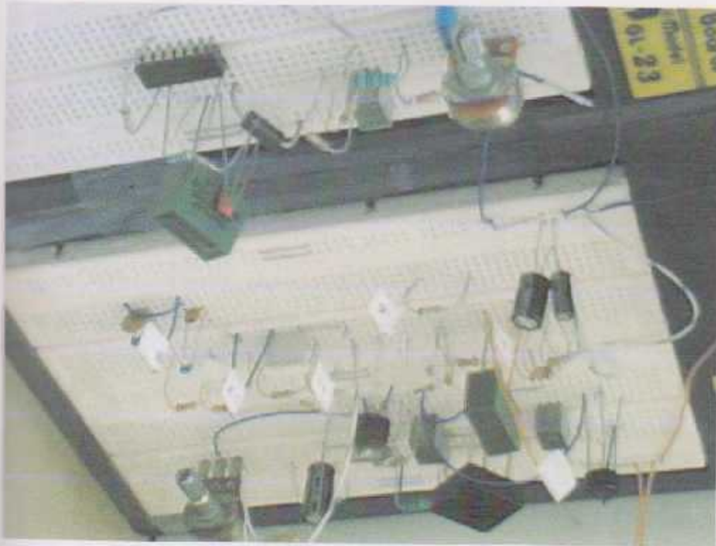
FIGURE 6.1 Temporary full circuit implementation on Bread Board
