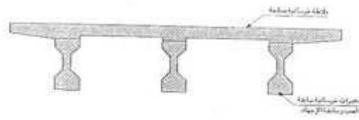
(C) PRECAST I - GIRDER BRIDGE
