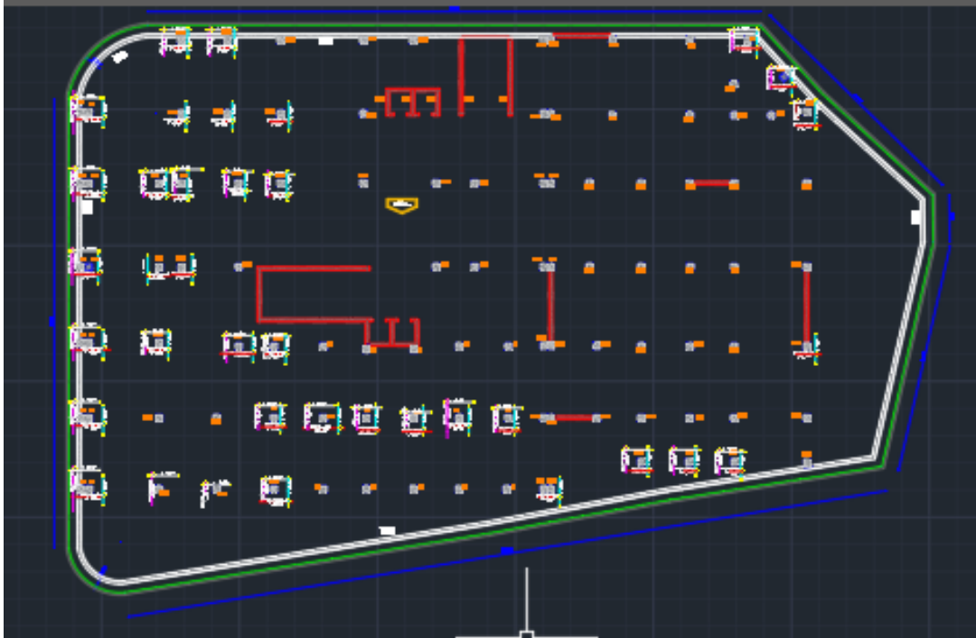
Figure (4-28) : Mat footing additional reinforcement .
