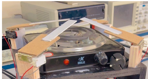
Figure 4.6: Limit Switches Installation
