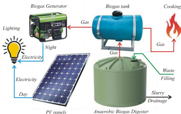
Figure 2. Hybrid energy unit, PV solar panels and anaerobic biogas digester
