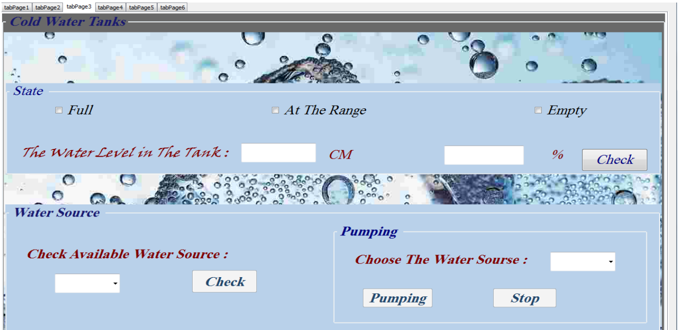
Figure (5.19) : PC Platform To Control and Manage Cold Water Tanks.
