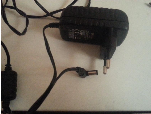
Figure(6.10) : GSM External Power Supply .
