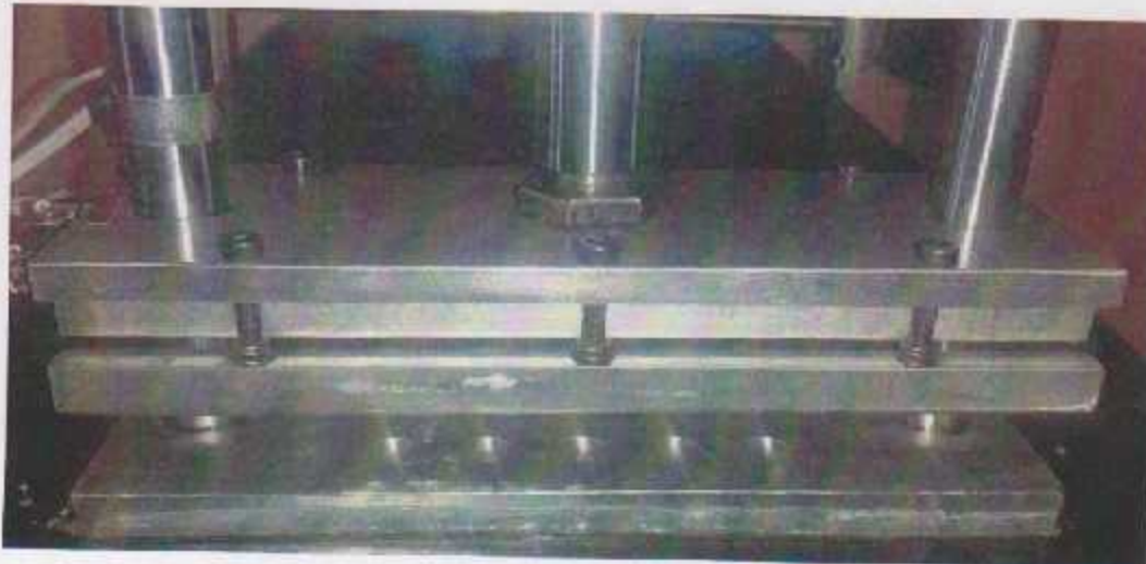
Figure 6.3. The template that works on the formation of aluminum foil
