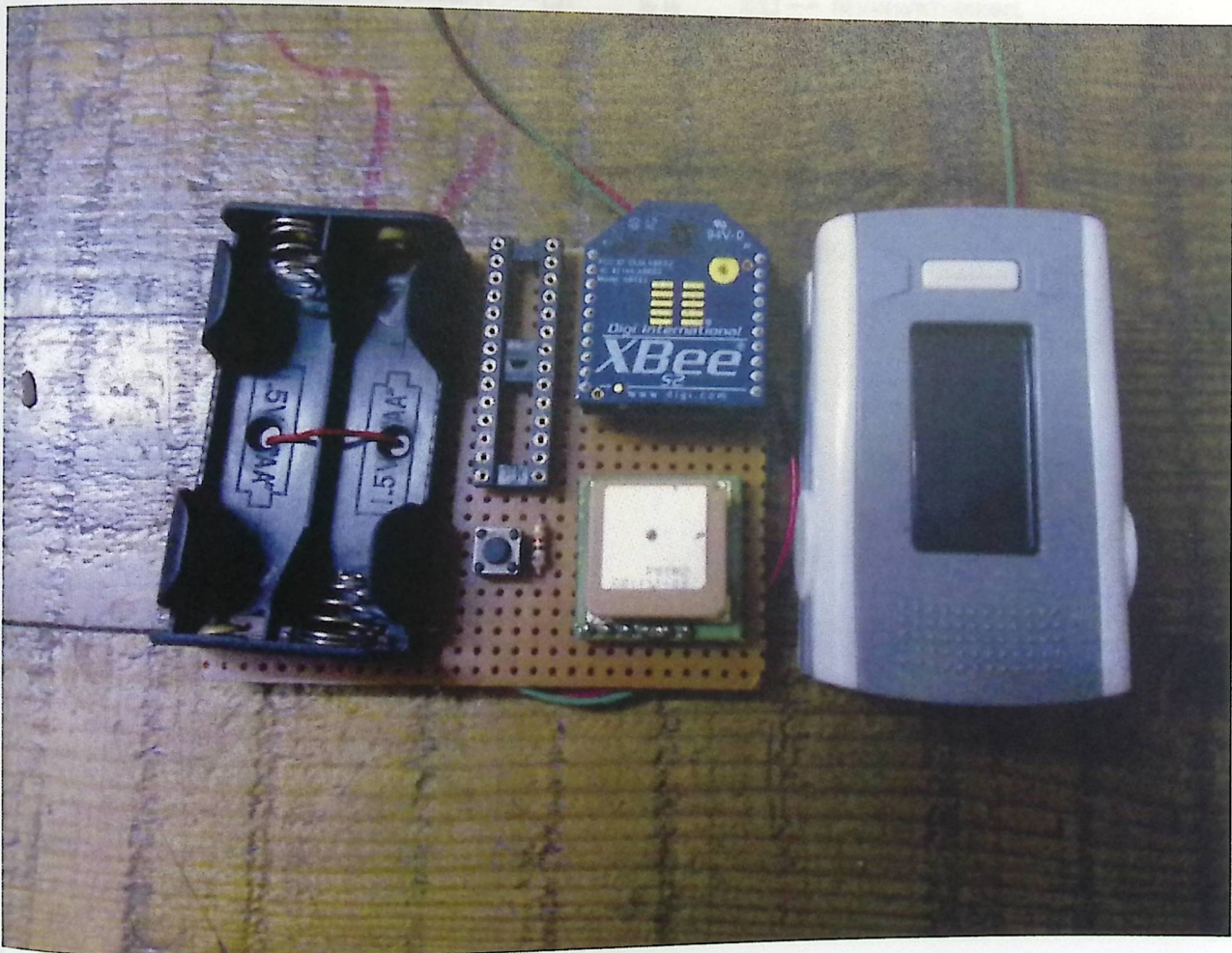
Figure 4.1 : transmitter side elements
