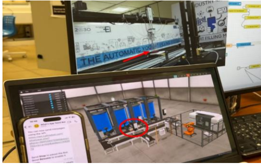
Figure 7 Synchronization between real and virtual systems
