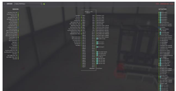
Figure 5 PLC driver in Factory IO
