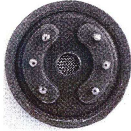
Figure 4.55 MQ3, bottom view
