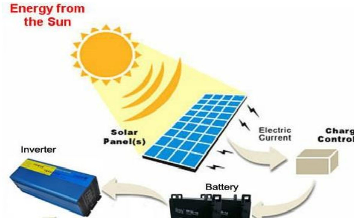
Figure 3.13: Parts of solar system.
