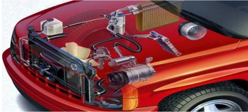
Figure 2.2: Vehicle air condition system
