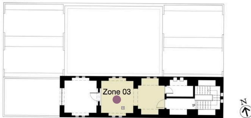
Figure 6-7: Location of the data logger in Zone 3 (marked by the circle), positioned at 1.2 m above floor level, on the first-floor plan (author's drawing).
