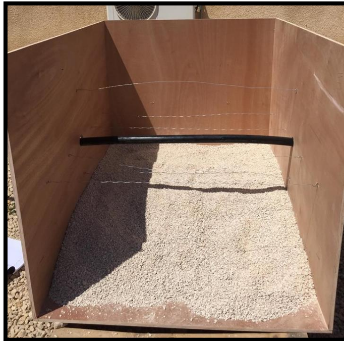
Fig (4.3) embedding the cable test into container
