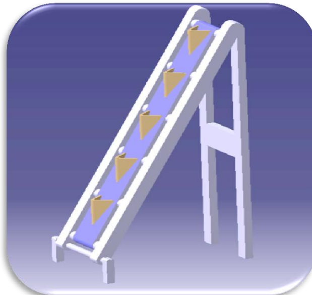
Figure (3.12): Lift conveyor.
