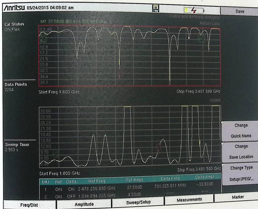
Figure 5.2.10: Measured Return loss vs. frequency of Optimum antenna with existing skin.
