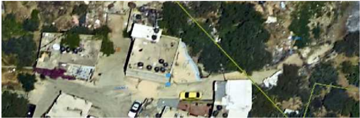
Figure ( . ) Relief Displacement in Buildings
