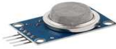
Figure2.3: MQ_2 gas sensor, source [10]
