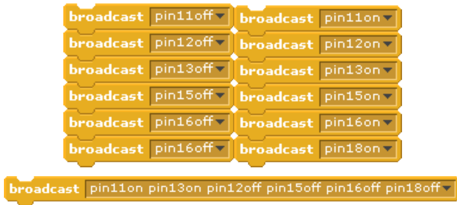
Figure 5.22: way of enabling and disabling GPIO pins
