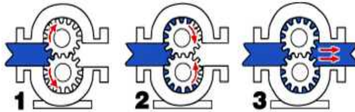
Figure 5.3: Principle of operation for gear/pump motor.
