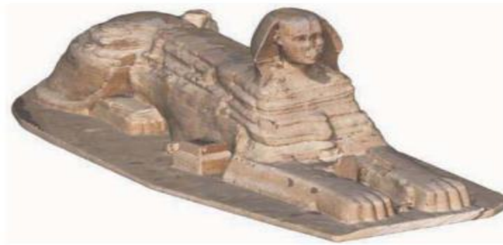
Figure (3-11): Triangulated point cloud of the Sphinx textured in Rican Pro, combined from seven scanner positions: six from the ground and one from the Cheops Pyramid.[14]
