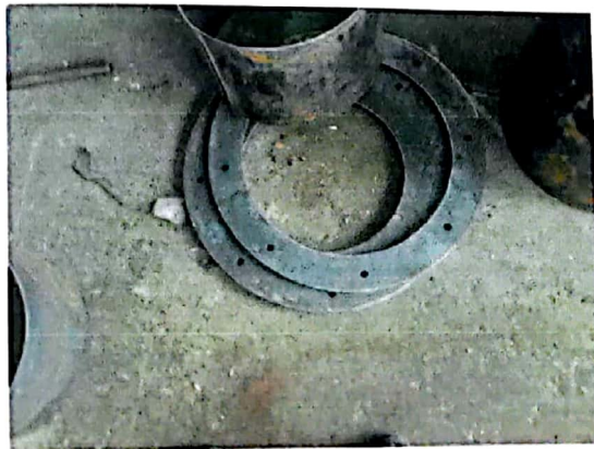
Figure (5.22) : Flanges drilling.
