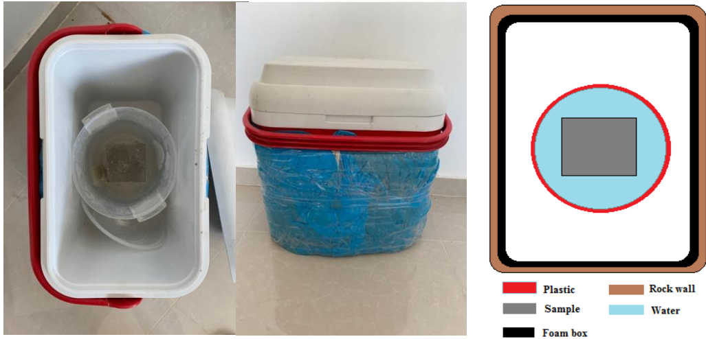
Figure 3.6: A homemade thermal calorimetric device for testing of specific heat.
