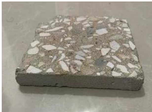
Figure 3.4: Optimum concrete thin specimen with a 1 cm thickness.
