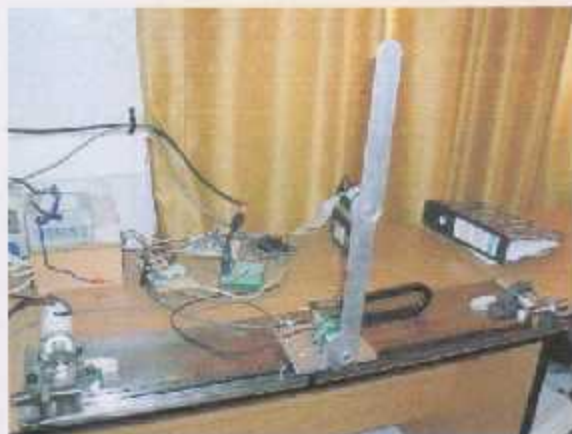
Figure 2 DIP system composed of two aluminum rods and a cart and actuated by an AC servomotor through a specially-designed rope-and-pulley mechanism
