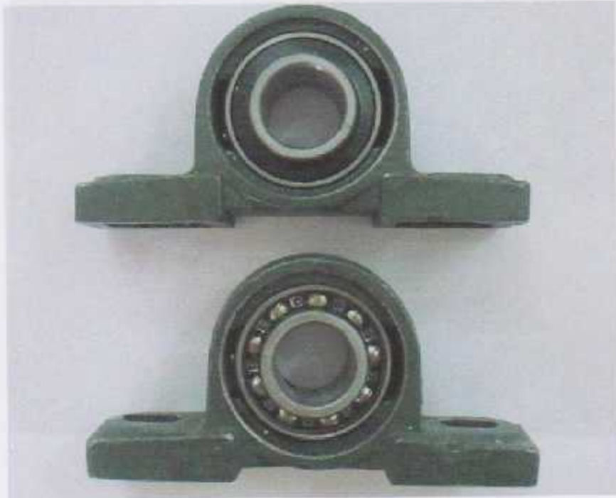
Figure A.2 Ball bearing before and after removing the lubricant and its keeper.
