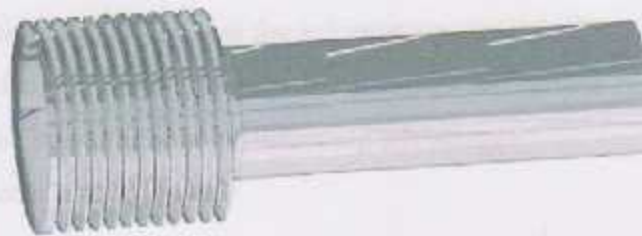
Figure 1.4 Helical pulley used for power transition from the motor to the cart.
