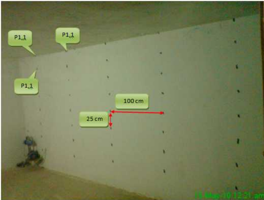
Figure 4.27: the distribution of points at the inner side of the wall of class 5.
