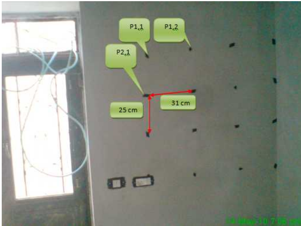
Figure 4.22: the distribution of points at the inner side of the wall in class 4.
