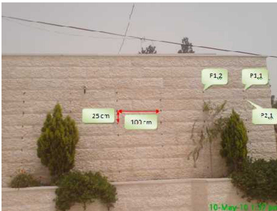
Figure 4.28: the distribution of points at the outer side of the wall of class 5.
