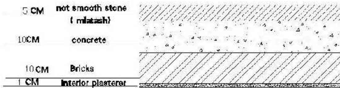
Figure 4.29: cross section of outer wall of class 12.[12]
