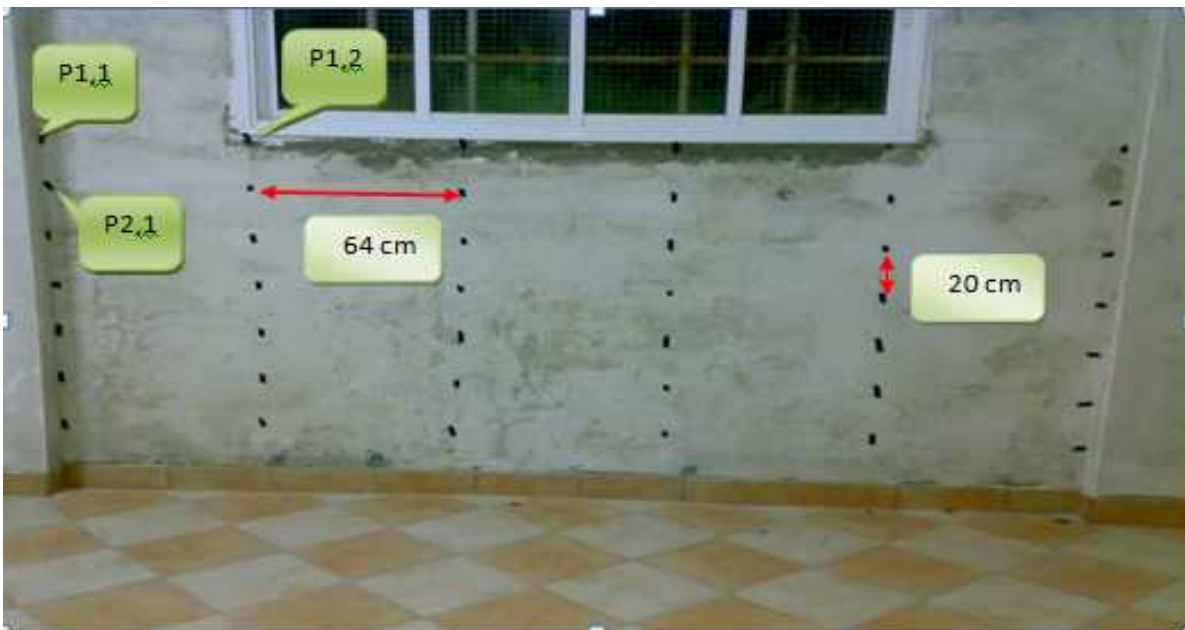
Figure 4.9: The distribution of points at the inner side of the wall in class 1.
