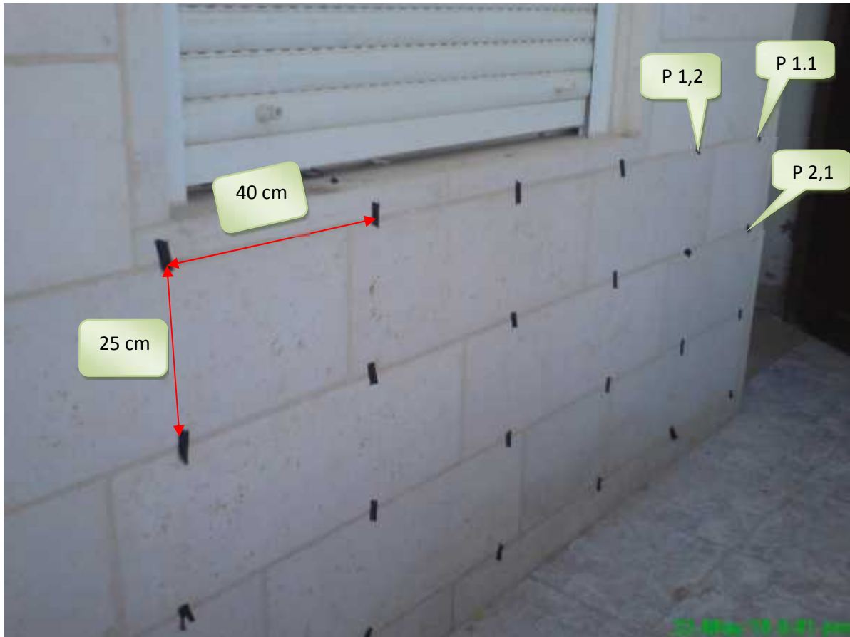
Figure 4.51: the distribution of points at the outer side of the wall in class 10.
