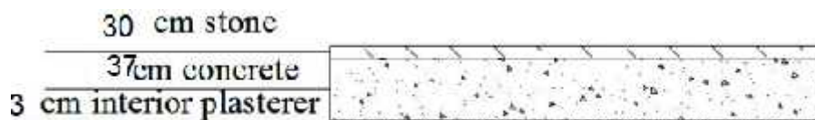
Figure 4.11: cross section of the outer wall for class 2.[12]
