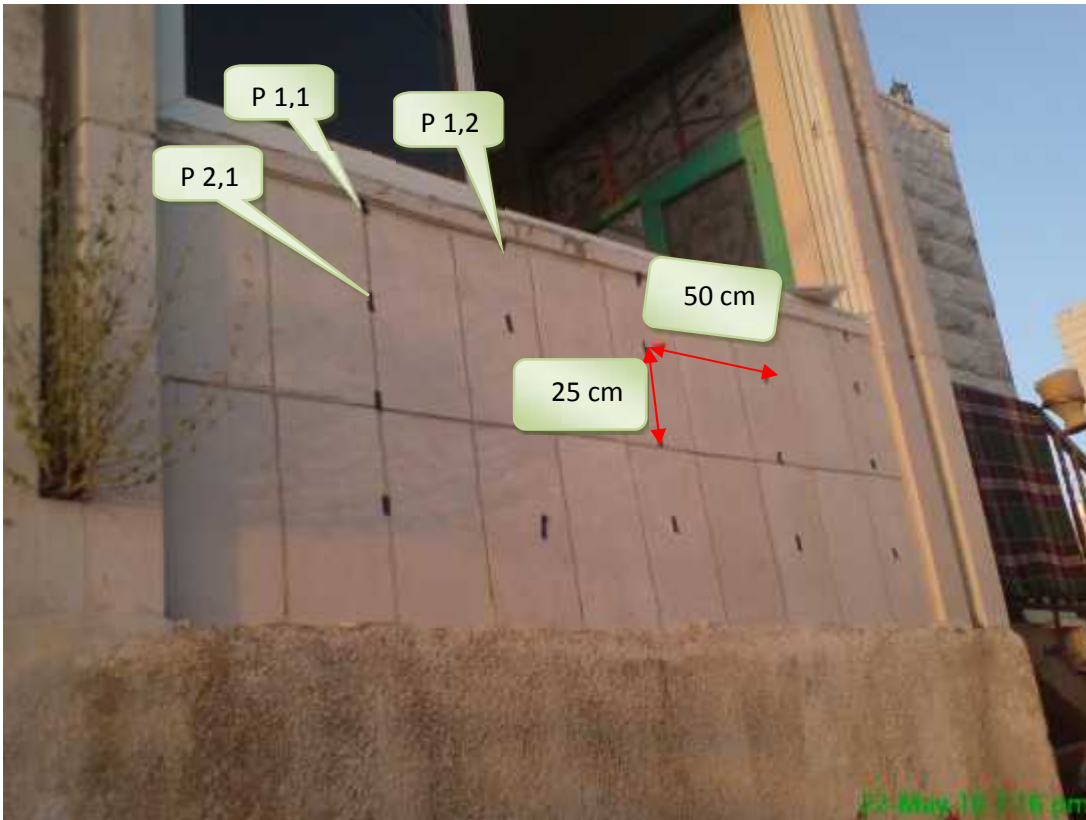
Figure 4.54: the distribution of points at the outer side of the wall in class 11.
