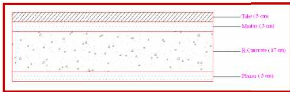
Fig.(4-32) Section in Stair's Landing
