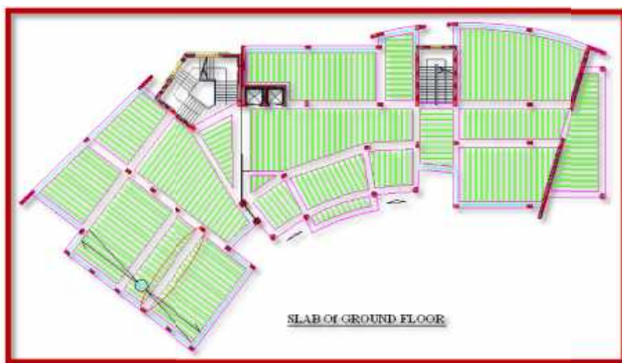
Fig.(4-3) Structural Key Plane
