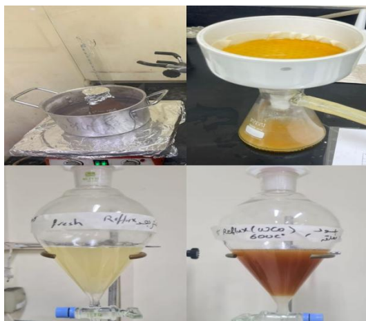
Figure 5: Biodiesel production steps
