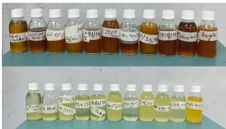
Figure 8: Biodiesel products obtained under various catalyst types and operating conditions, from left to right: NaOH; dried eggshell (105 °C) at 10 g for 1 and 2 h; dried eggshell (105 °C) at 2 g and 18.18 g; room-temperature eggshell (25 °C); calcined eggshell (900 °C) at 10 g, 2 g, and 18.18 g; refluxed eggshell (600 °C) at 10 g; and recycled calcined eggshell
