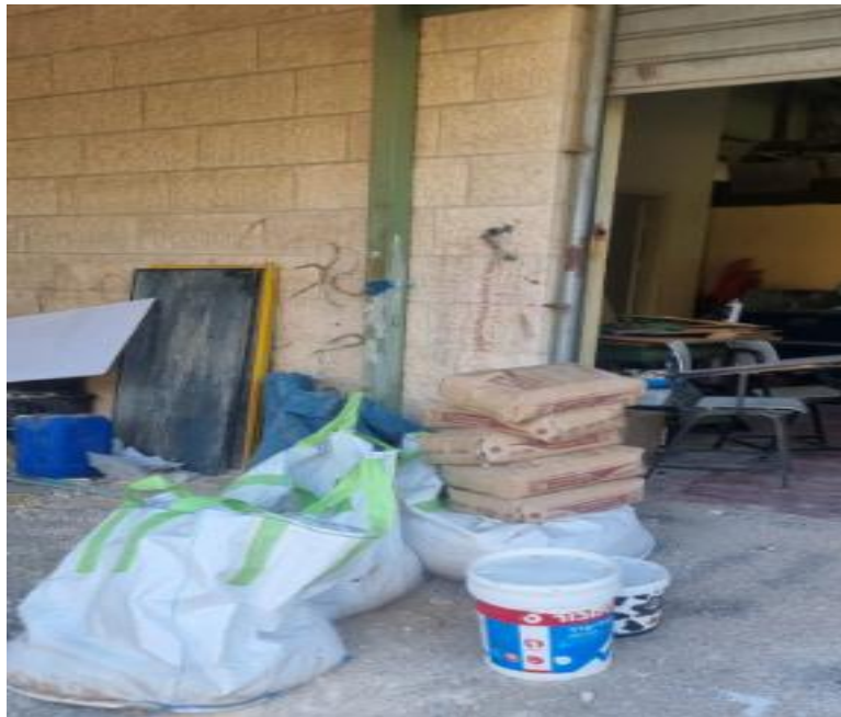
Figure 3. 1 : Locally sourced Nesher Cement (CEM I 42.5N) used as the primary binder during the experimental phase.
