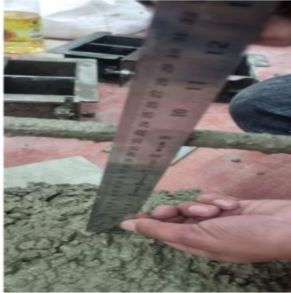
Figure 3. 5. Measurement of fresh concrete workability utilizing the standard slump test.
