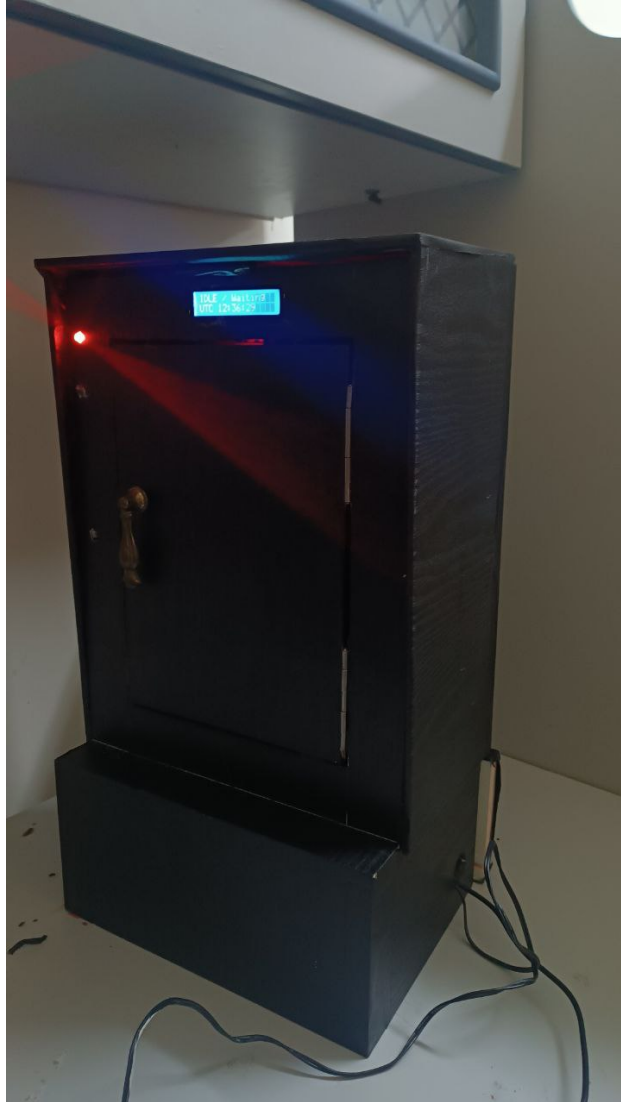
Figure 4.4: LiPass hardware prototype showing the secured door enclosure with integrated LEDs, LCD, photodiode, and Raspberry Pi.
