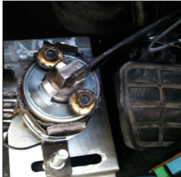
Figure 5.9: Brake solenoid installation
