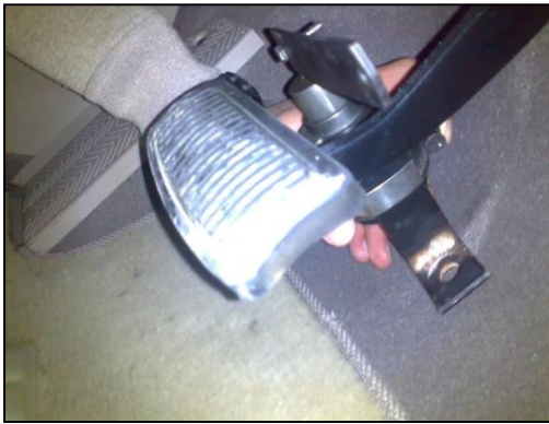
Figure 4.29: Brake actuator installation
