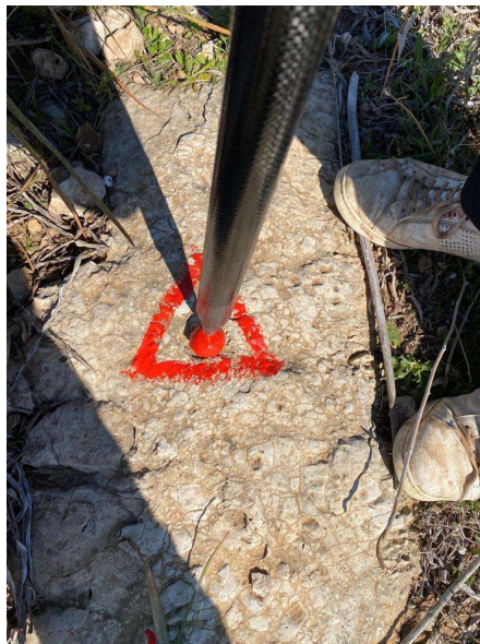
(a) Survey pole centered on the mark
