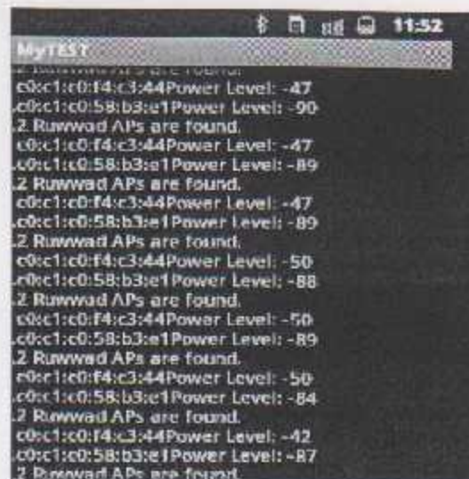
Figure 4.8: Example of the readings that were taken by the Mobile phone
