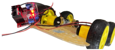
Figure 4.3: Motor Driver Positioning on the Chassis.
