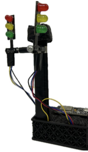
Figure 4.9: Traffic Light Setup with Microcontroller Base.
