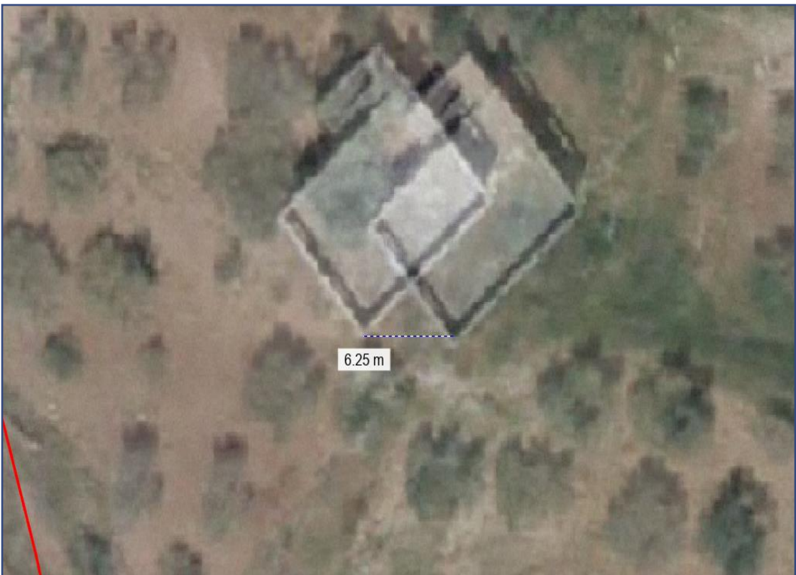
Figure 5- 10 : Displacement distance between the georeferenced orthophoto and original orthophoto
