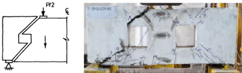
Figure 1. 3: Failure of reinforced concrete deep beams: (left) from Mansur and Alwis (1984); (right) from Jasim et al. (2020).
