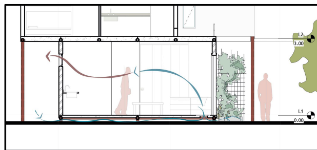
CROSS SECTION SHOWING A FLOOR OPENING ALLOWS COLD AIR TO FLOW FROM UNDERGROUND INTO THE SHELTER CREATING AIR CIRCULATION
