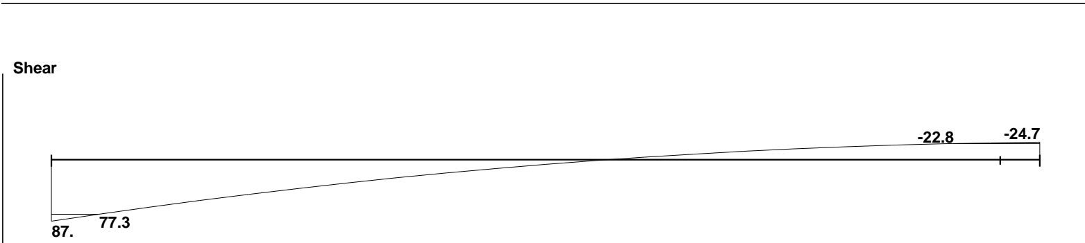
Fig 4.12: Shear and Moment Diagram for Basement Wall.
