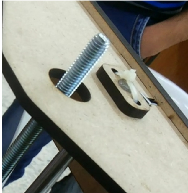
Figure 4.23 Threaded and smooth rods upper end
