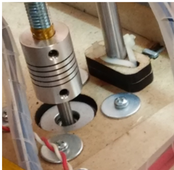
Figure 3.20 5/8mm Aluminum coupler on motor shaft
