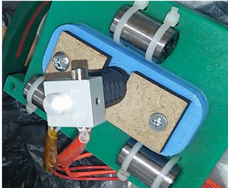
Figure 4.34 bearings under extruder
