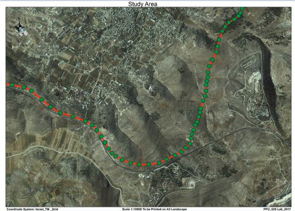
Figure B.3: Transmission line path-section(3)
