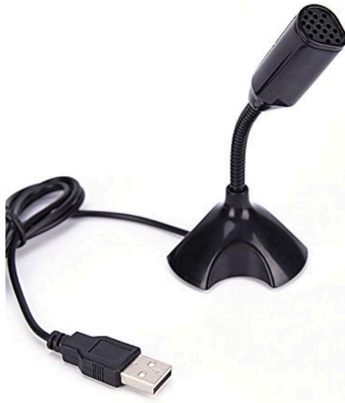
Figure 3.6: SR-ULM10 USB Microphone [15]
