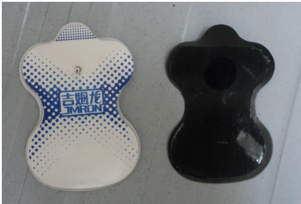
Fig. ( 3-43 ) Pre-gelled electrode
