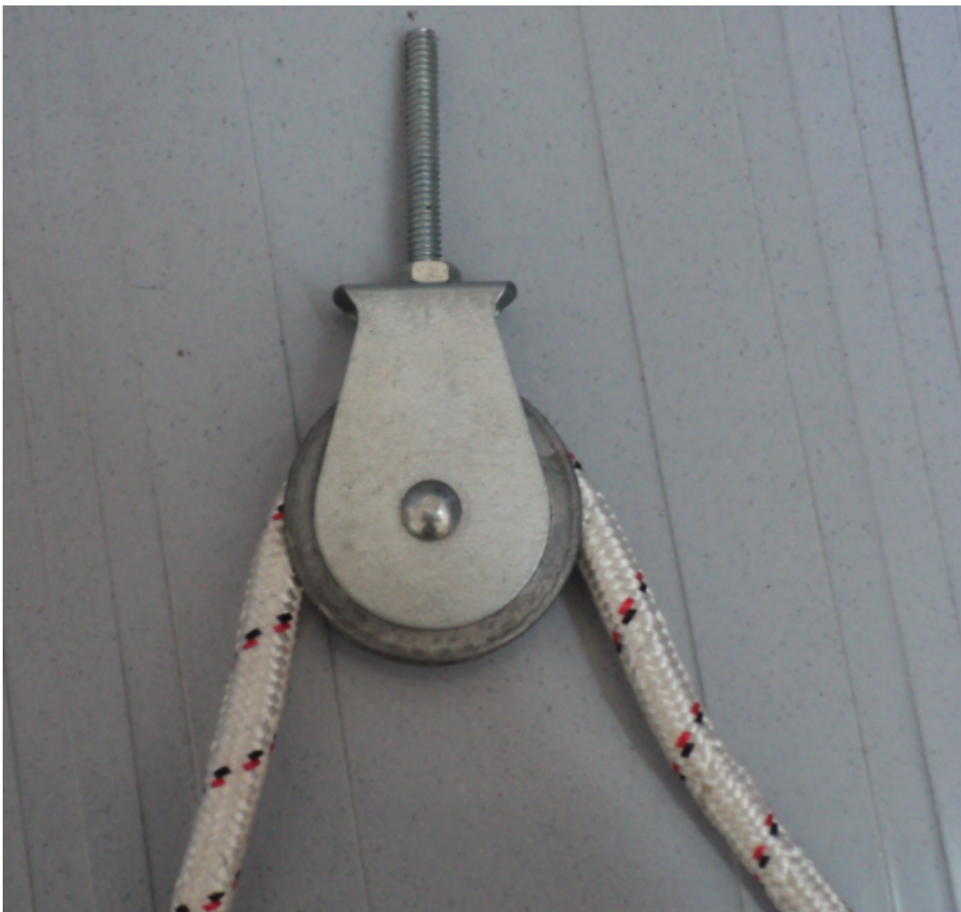
Fig.(3-14) Pulley System
