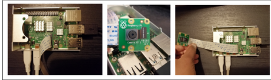
Figure 2.5: Pi camera and Raspberry Pi [4].
