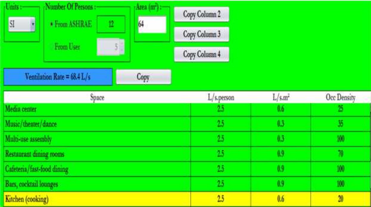
Figure 6: Calculation the Ventilation by program for kitchen
