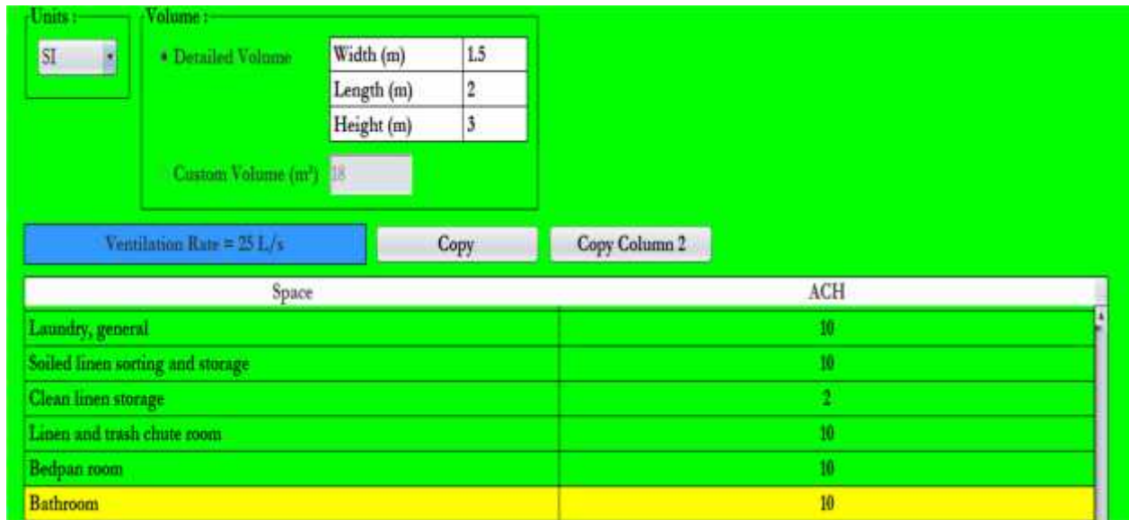
Figure 7: Calculation the Ventilation by program for bathroom
