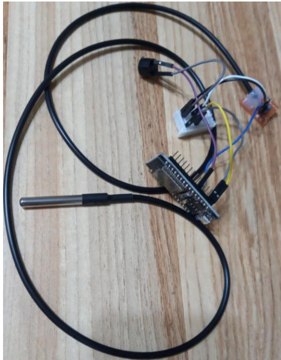
Figure 22: hardware (esp32 connect DS18B20 )
