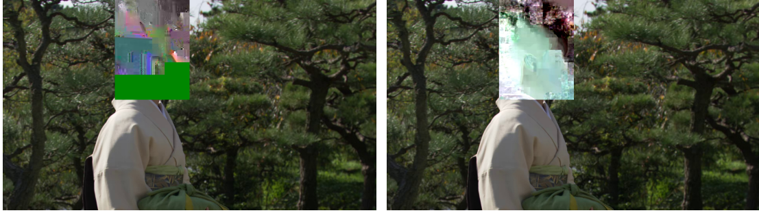
(a) TNE-HEVC PSNR1=10.95, PSNR2=42.07, (b) TSE-HEVC PSNR1=7.78, PSNR2=42.07, PSNR3= 21.15(dB) PSNR3=18.01 (dB)
